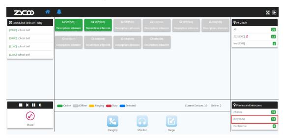
The control panel options of Intercom extensions including HangUP, Monitor and Barge. It's the same as control panel of IP phone extensions.
